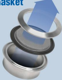
The Rubber Fab V2B Vent Gasket provides vacuum and pressure relief for **pharmaceutical** and **food/beverage processing** tank venting when **airborne particulate removal is required**. A 200 mesh screen combined with a 14 mesh screen of **sintered construction** creates a cost effective alternative to expensive vacuum breakers and venting systems.
